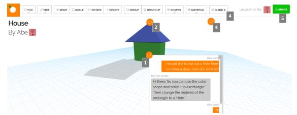
Fig. 1. MarmalAid user interface: (1) users can anchor chat windows to request remote assistance on any part of their model; (2) by clicking on the comment icon, the chat window collapses but remains attached; (3) document-level chat windows can also be added without a model-specific anchor; (4) the Q and A icon is used to create a new chat window; (5) the Share feature can be used to obtain a model-specific URL for sharing.
